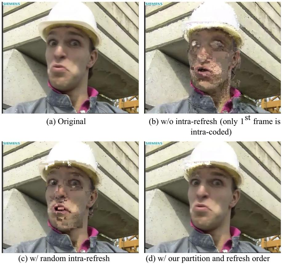
Fig. 10. One reconstructed frame from “foreman” with transmission error. In different methods, the lost frames are the same.
