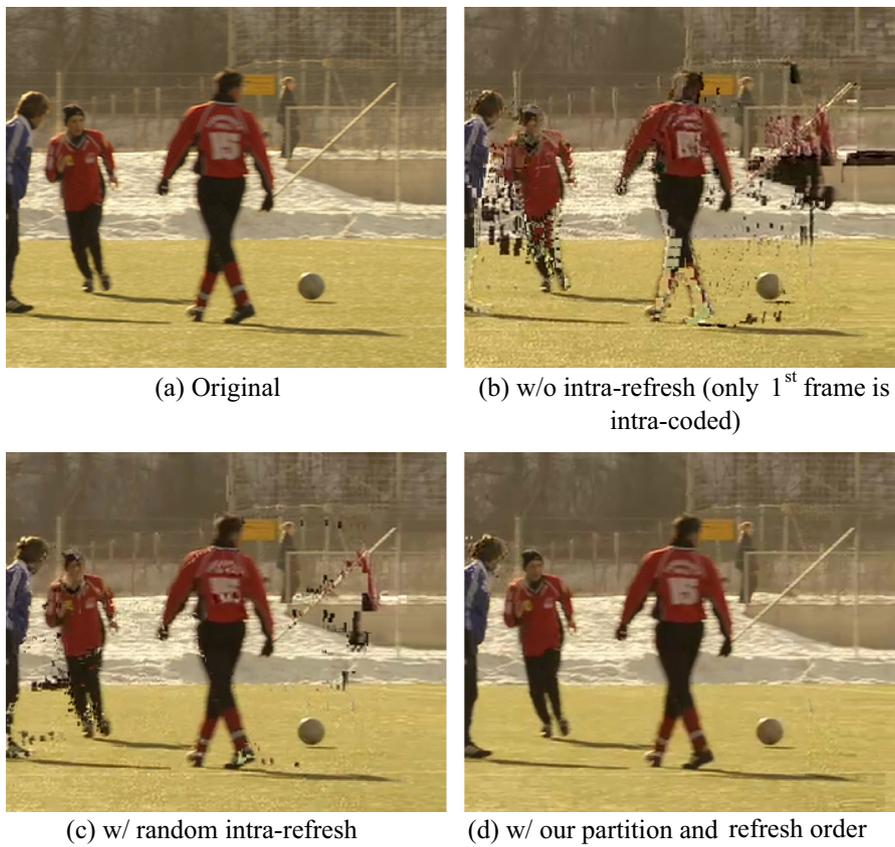
Fig. 11. One reconstructed frame from “soccer” with transmission error. In different methods, the lost frames are the same.
