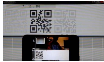
Fig. 5. A video frame showing the QR codes with a space diversity of four.
