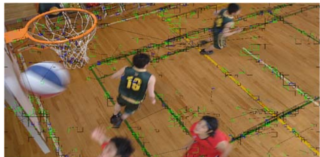
Figure 6. Different types of IntraBC-coded blocks in a frame in “BasketballDrill”. Black is the current block being coded. (Blue: Fractional IntraBC, green: Boundary Matching IntraBC, red: Regular IntraBC. Best view in color).
