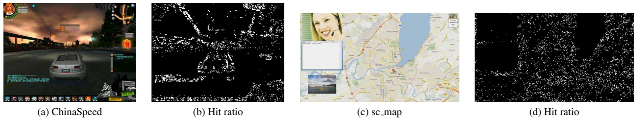
Fig. 4. First frames of two video sequences: ChinaSpeed and sc_map, and their corresponding hit ratio illustration. The white blocks denote the 4 \times 4 blocks using NN interpolation, and the black blocks use bilinear interpolation, or are IntraBC blocks (Figure best viewed in color.)
