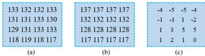
Fig. 3. Example of a  $4 \times 4$  block predicted by the horizontal mode (mode 10). (a) Original block. (b) Prediction block. (c) Residual block.
