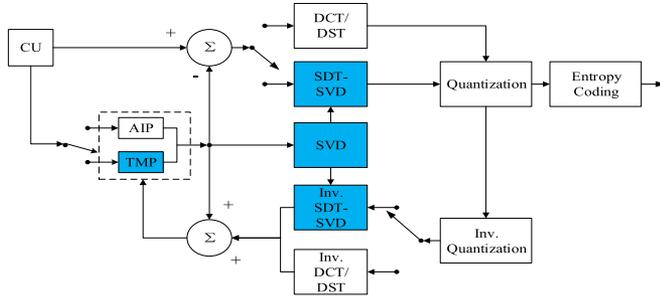
Fig. 5. Framework of intra coding with the proposed SDT-SVD. The blue boxes are new added parts for the proposed coding method.
