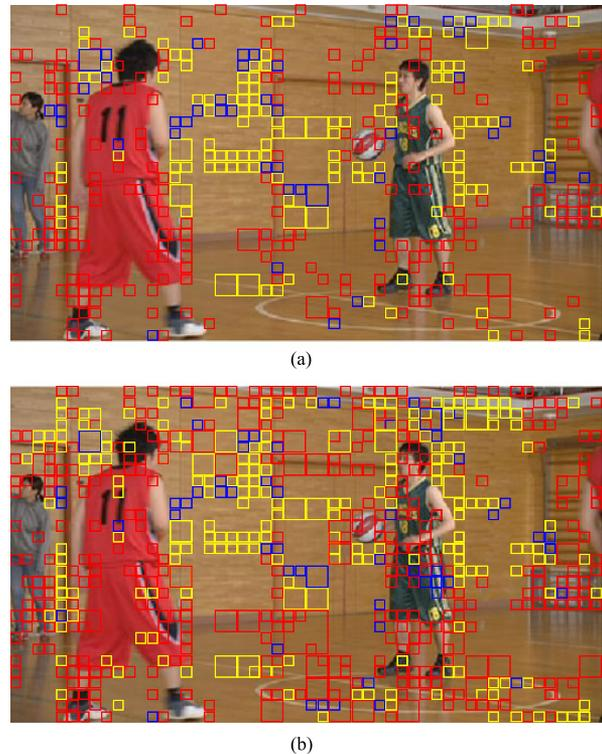
Fig. 11. Modes distributions for the first frame in sequence *BasketballPass*. The blocks marked with red boxes are coded by AIP with SDT-SVD, the blocks marked with yellow boxes are coded by TMP without SDT-SVD, and the blocks marked with blue boxes are coded by TMP with SDT-SVD. Other regions except these blocks with colored boxes are coded by original intra coding in HEVC. (a) QP = 22. (b) QP = 32.
