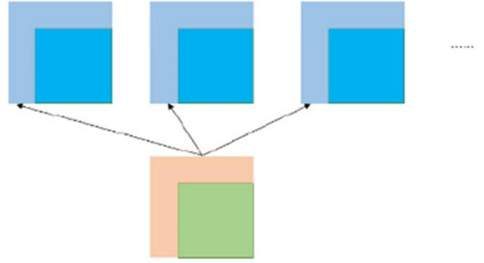
Fig. 7. Template matching process. Inverse-L area is the template (in light blue) used in the matching process. All the deep blue blocks are the prediction candidates for the current block (in green).
