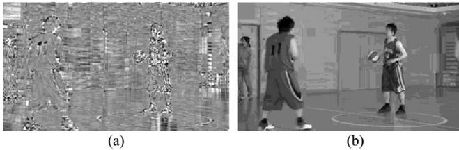
Fig. 2. (a) One residual frame (shown with enhanced contrast and best viewed when zoom in) and (b) the corresponding prediction frame from sequence *BasketballPass* by HEVC intra coding when  $QP = 22$ . (a) Residual frame. (b) Prediction frame.
